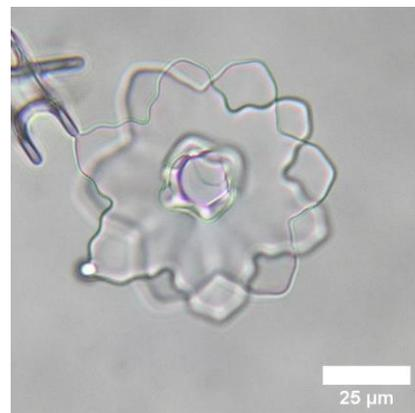
図1 人工十二花結晶 ( $\phi$ :26.6°)
