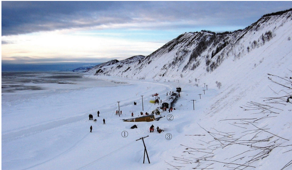
Fig. 1. Train derailed by an avalanche on 31 Dec. 2009, eastern coast of Sakhalin Island (219 km from Korsakov along the Korsakov-Nogliki railway). Numbers correspond to buried machinery: 1 & 2: locomotive and snow-cleaning car hit by the first avalanche, respectively; 3: breakdown gang's bulldozer hit by the second avalanche.
