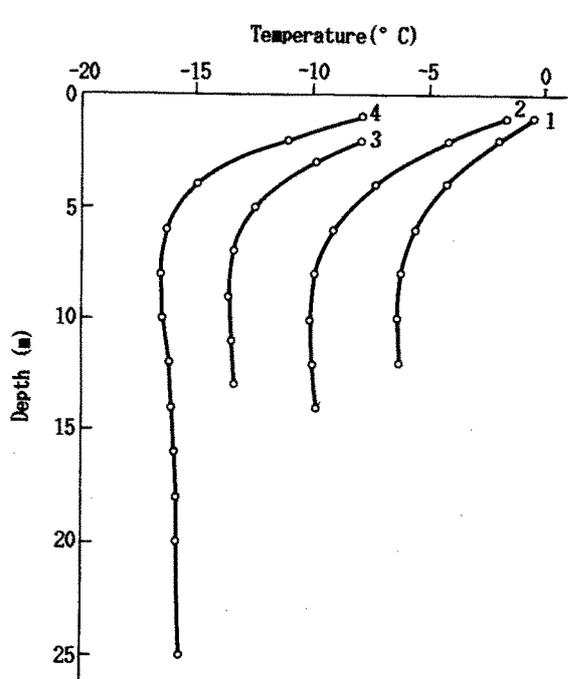
Fig. 2. Measured temperature profiles in boreholes on Chongce Ice Cap and Guozha Glacier on Aug. 26, 1987.
