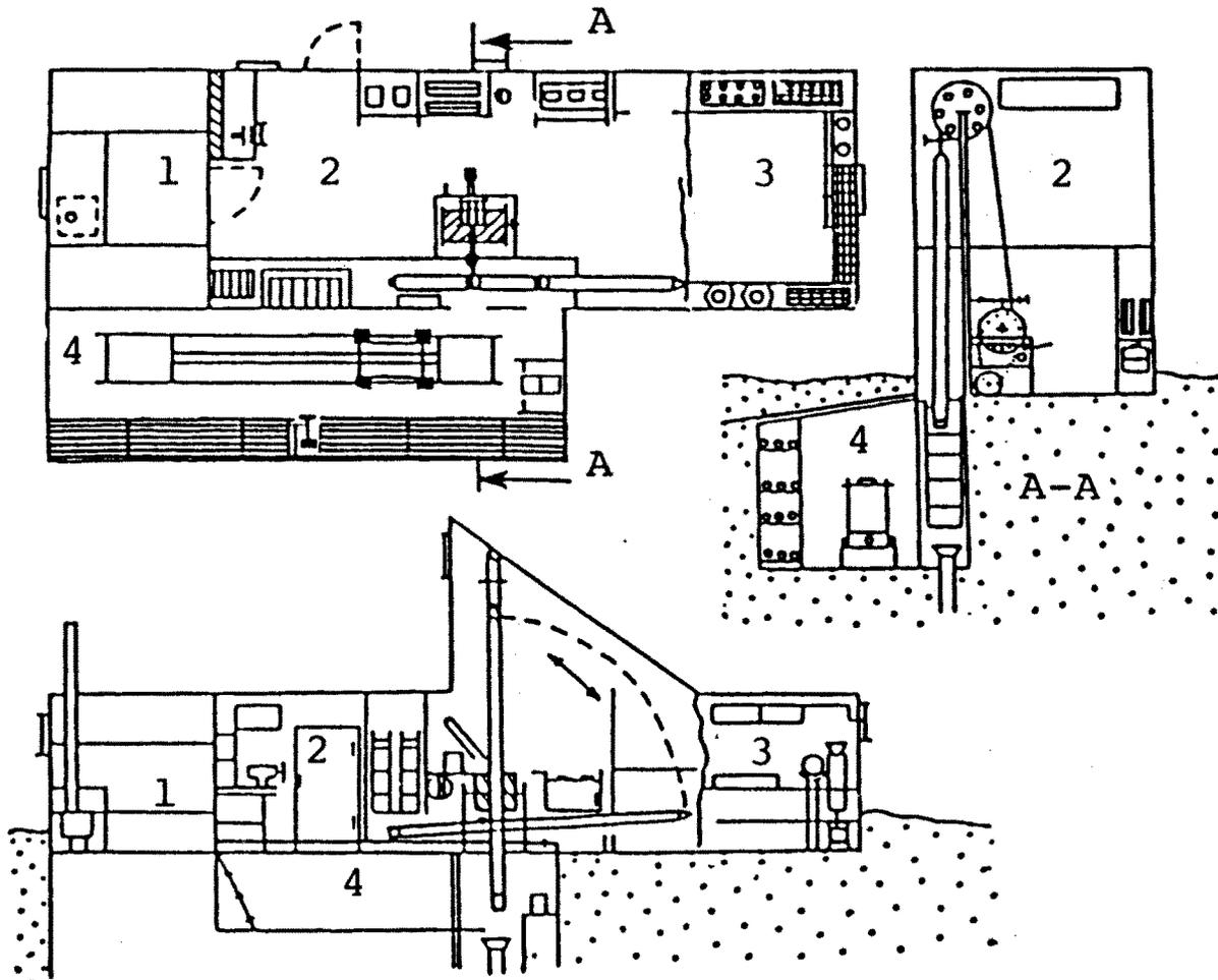
Fig. 1. Drilling complex. 1 : residential block, 2 : drilling chamber and laboratory for structural studies of ice core, 3 : geochemical laboratory, 4 : cold laboratory / ice core warehouse.
