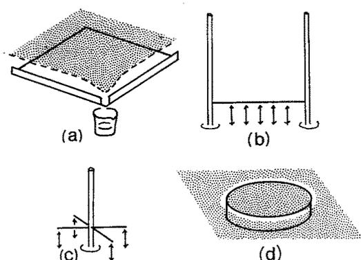
Fig. 3. Methods for melting rate observation. (a) lysimeter, (b) two stakes with a strained string, (c) stake with four horizontal sticks, (d) evaporation pan in which melt water was weighed.
