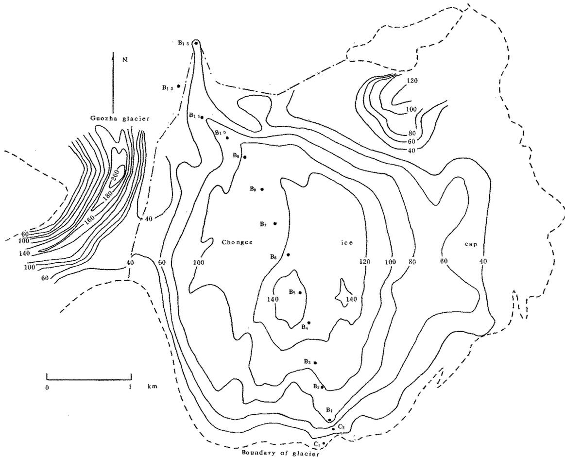
Fig. 6. Isopach of the ice thickness of the Chongce Ice Cap
