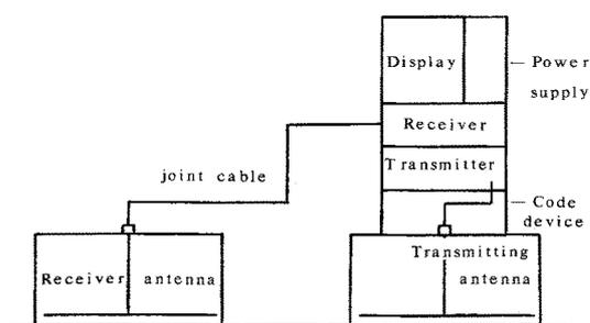
Fig. 2a. Diagram of the improved version of type B-1 radar.
