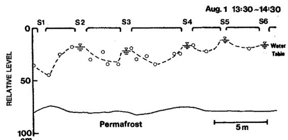
Fig. 11. Surface flow, and water table and permafrost table for the experimental cross section, near ABC on August 1, 13: 30–14:30. S1 – S6 shows sections of stone boulder.
