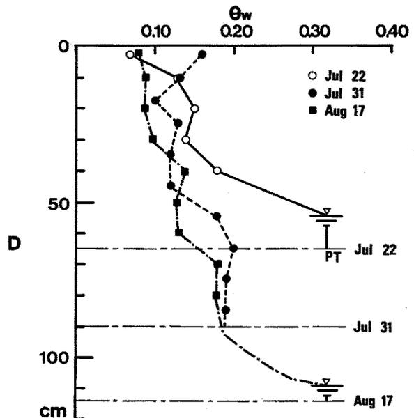
Fig. 10. Soil moisture observed by pit at ABC on July 22 and 31, and August 17. P.T. stands for permafrost table.
