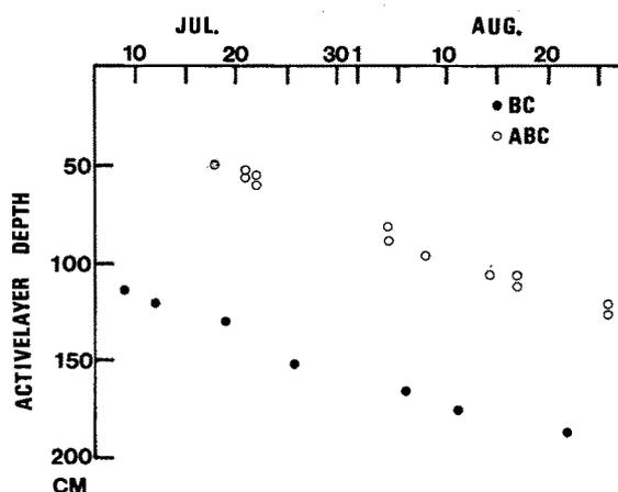
Fig. 2. Change of thawing depth of permafrost layer at BC and ABC for the observation period.
