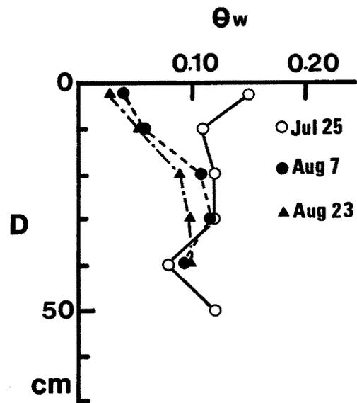
Fig. 7. Soil moisture in volume content ( $\theta_w$ ) for 0 - 45 cm depth (D) at BC.
