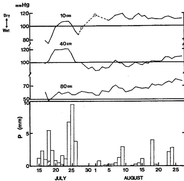
Fig. 6. Variation of soil moisture tension and precipitation (P) at BC.
