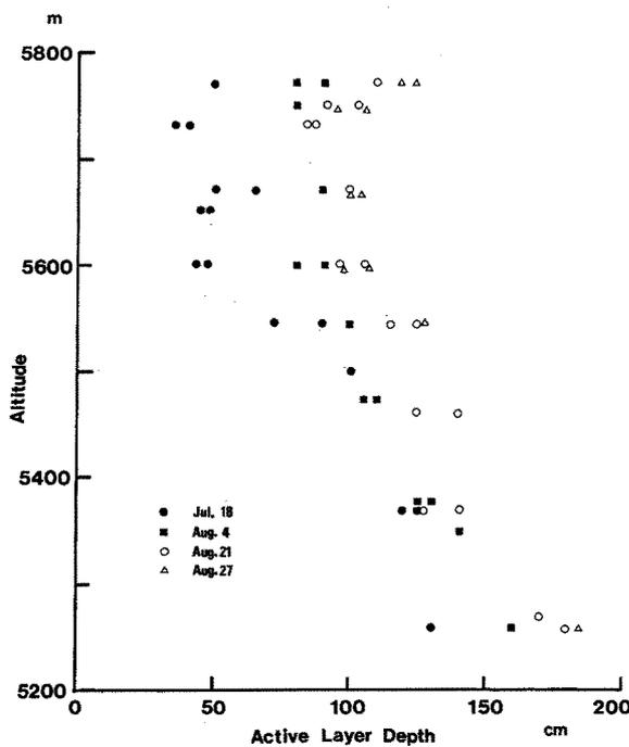
Fig. 4. Altitudinal variation of thawing depth for four dates.
