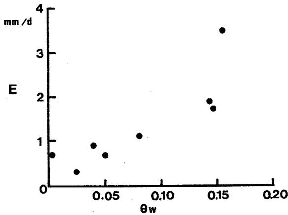
Fig. 8. Relation between daily evaporation (E) and soil moisture ( $\theta_w$ ) at 0 – 5cm depth.
