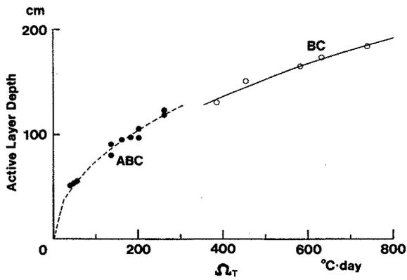
Fig. 3. Relation between thawing depth ( $Z$ ) and accumulated daily mean surface temperature ( $\Omega_T$ ) at BC and ABC.
