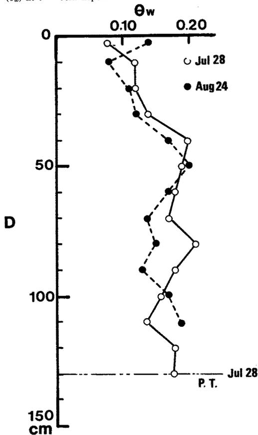
Fig. 9. Soil moisture observed by pit at BC on July 28 and August 24. P.T. stands for permafrost table.
