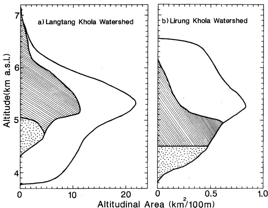
Fig. 3. Altitudinal distributions of the area of watersheds and glaciers every 100m in altitude. Dotted and hatched areas respectively represent the parts of debris-covered glaciers and debris-free glaciers.
