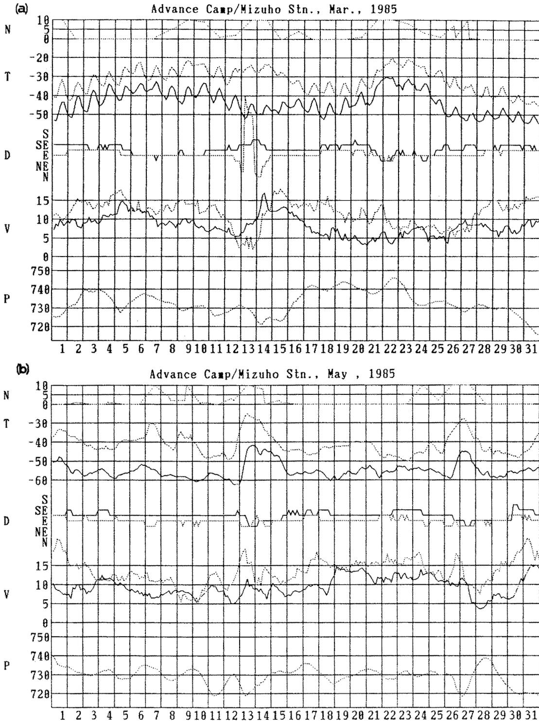
Fig. 3. Meteorological data from Advance Camp (solid lines) and Mizuho Station (dotted lines), (a) March, (b) May, (c) July, and (d) December, 1985. *N* is the cloud amount in the tenth scale, *T* the air temperature in °C, *D* the wind direction, *V* the wind speed in  $\text{m s}^{-1}$  and *P* the atmospheric pressure at the station level in hPa.
