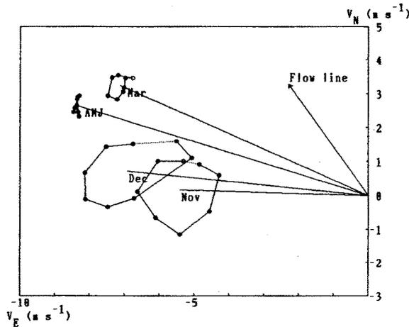
Fig. 4. Daily cycle wind vector variations at Advance Camp for March, April-May-June (combined), November and December, 1985. Open circles denote 3 LT data and dotted lines connect 24 to 3 LT.  $V_N$  and  $V_E$  denote northward and eastward components, respectively, of the wind vector. 'Flow line' indicates the surface slope direction.
