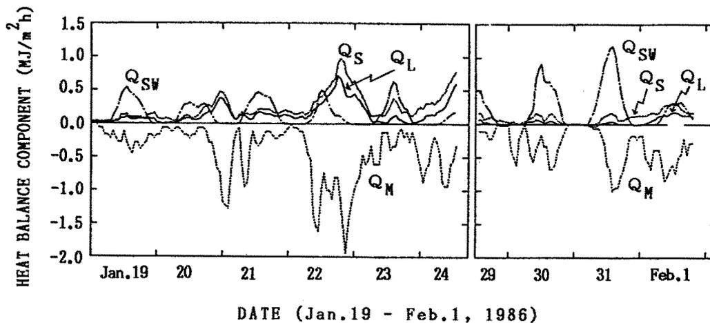
Fig. 3. Three-hour running mean of hourly effective shortwave radiation, sensible heat flux, latent heat flux and heat used to melt snow.
