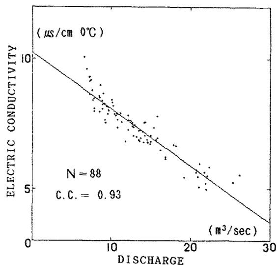
Fig. 5. Relation of discharge to electrical conductivity in the Cacho River.
