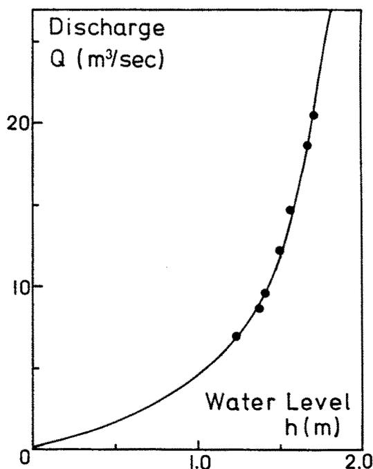
Fig. 2. Relation of discharge to river water level (stage-discharge curve)
