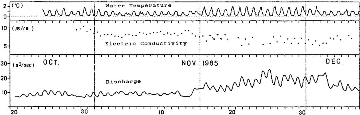
Fig. 4. 3-hourly variation of discharge, water temperature and electrical conductivity in the Cacho River.
