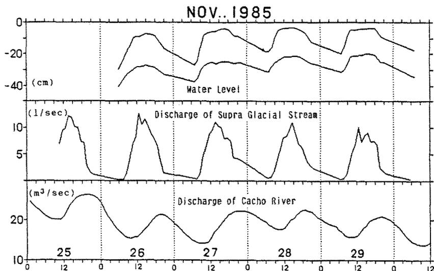
Fig. 6. Hourly variation of water level in surface ice body, discharge in supraglacial stream on Soler Glacier and discharge in the Cacho River, November 25-30, 1985.
