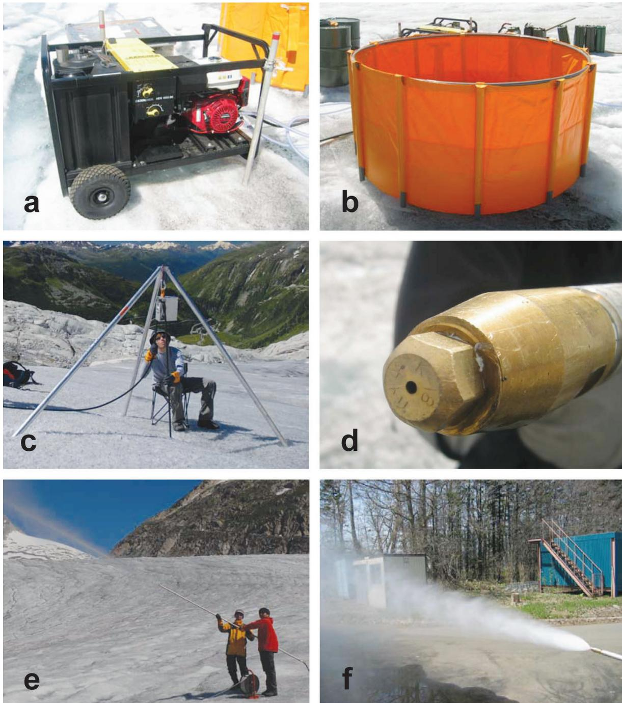
Fig. 3. (a) The high-pressure hot water machine (Kärcher HDS1000BE), (b) the 3000 l water basin, (c) the tripod with its pulley, (d) a jet nozzle mounted at the tip of the drilling stem, (e) a water jet from a 3 m long drilling stem with a straight nozzle, and (f) a water jet from the conic spray nozzle.
