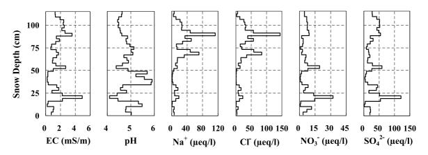
Fig. 5. Vertical profiles representing electric conductivity, pH, and major ion concentrations in snowpack samples.
