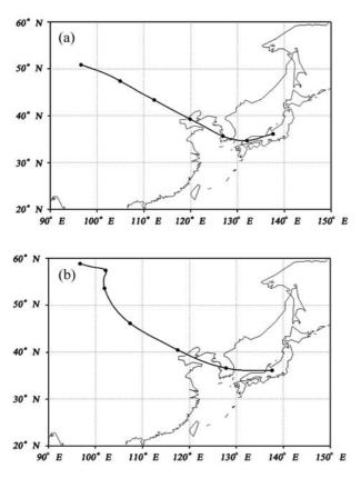
Fig. 11. Air mass back-trajectory generated using the CGER-METEX model for winter precipitation observed at sampling site. • denotes every 12 h. (a) Low-pressure system that passed the vicinity of Japan ending on February 6, 2007, at 10:00 (JST), (b) Winter monsoon pattern ending on February 8, 2007, at 9:00 (JST).
