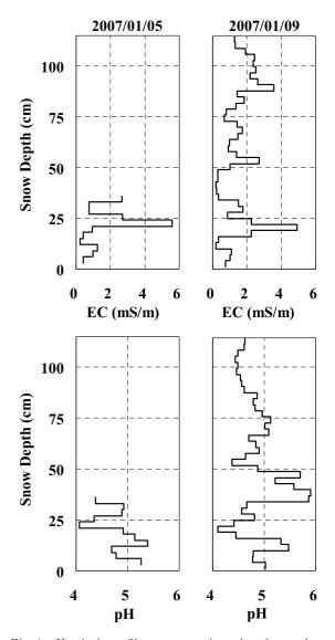
Fig. 4. Vertical profiles representing electric conductivity and pH in snowpack samples obtained on January 5 and January 9, 2007.
