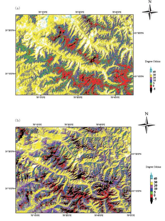
Fig. 6. Distribution patterns of the effective temperatures derived from the ETM+ band 6 (Low gain) scenes for 02-June-2000 (a) and 08-October-2000 (b).
