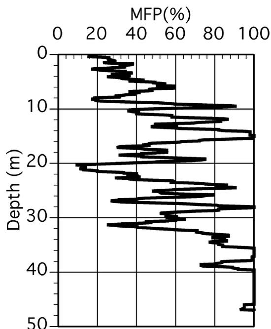
Fig. 7. Profile of the melt-feature percentage (MFP) in the ice core. MFP indicates the proportion of ice layers in 1-m-long sections of the ice core, measured at 0.1-m intervals.
