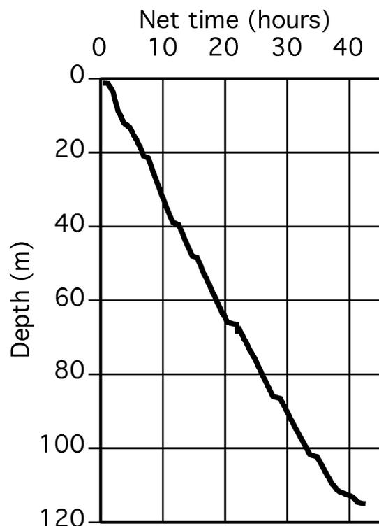
Fig. 4. Cumulative drilling time (h) versus depth (m).
