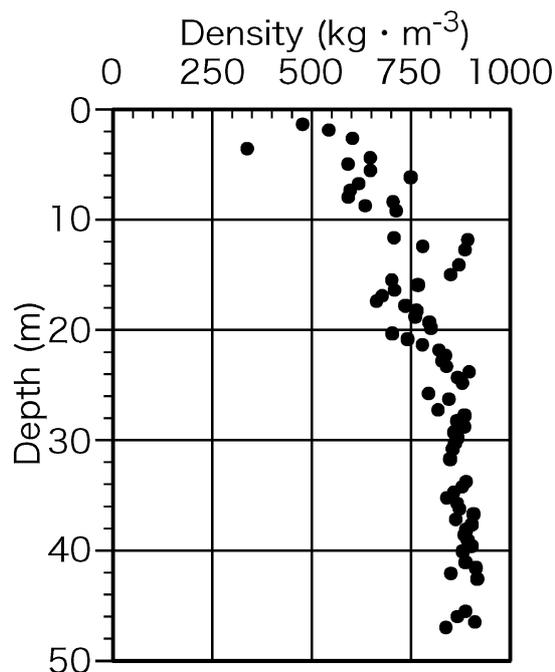
Fig. 6. Bulk density profile of the ice core from the surface to 50 m depth.
