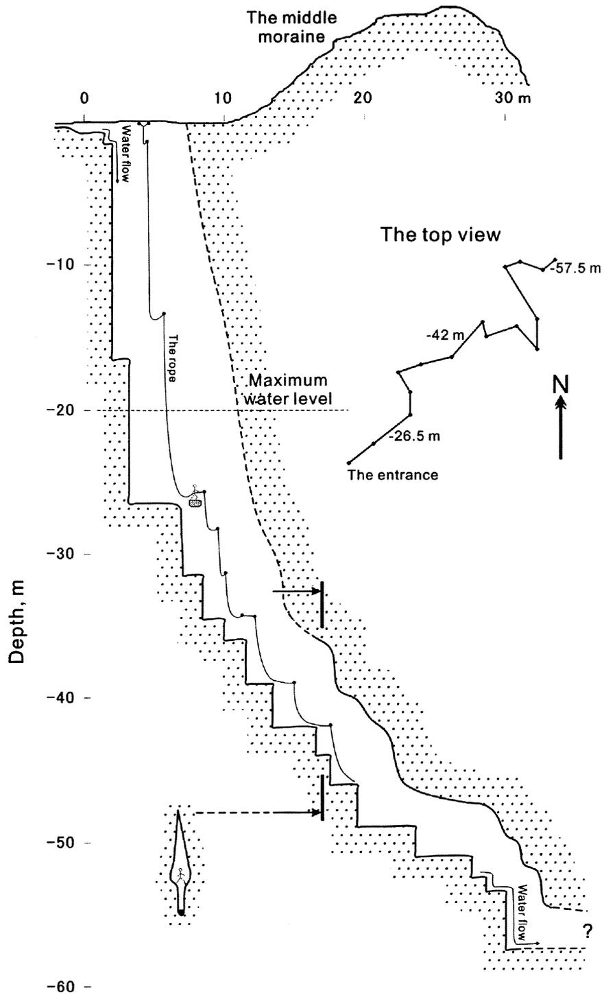
Fig. 6. The map (profile sweeping and top view) of the moulin B. The right boundary and the ceiling of the upper part of the moulin are unclear, that illustrated by the dashed line.
