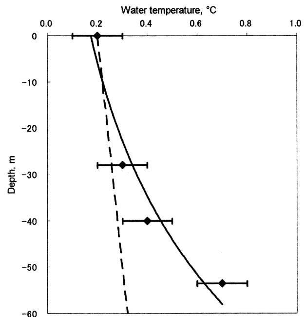
Fig. 7. Vertical profile of water temperature in the moulin B. The maximum rate of water temperature increase, estimated by the loss of potential energy, is shown by the dashed line.
