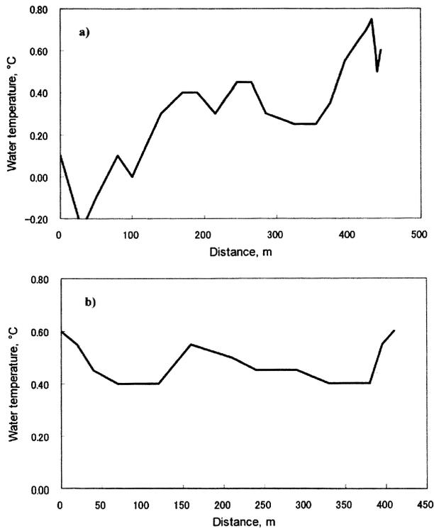
Fig. 4. Water temperature profile along surface water streams. a) at the upper part of the ablation area; total length 445 m, discharge from 2–3 to 50 l s<sup>-1</sup>. b) near the terminus; total length 410 m, discharge from 3 to 30 l s<sup>-1</sup>.
