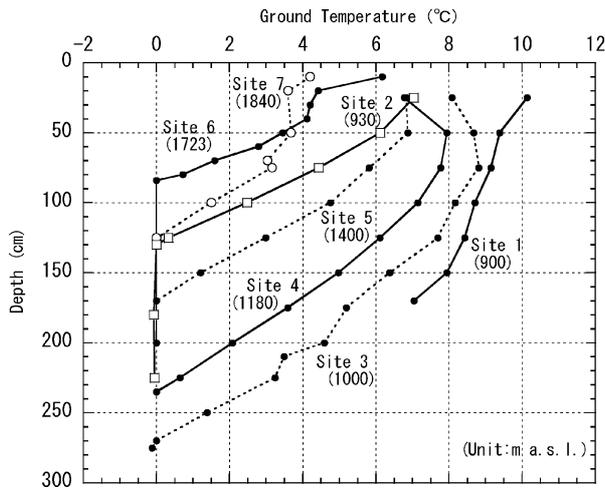
Fig. 2. Ground temperature profiles for sites on Mt. Ichinsky, as measured from August 26 until September 1, 2000. Site elevations (m.a.s.l.) are also provided.
