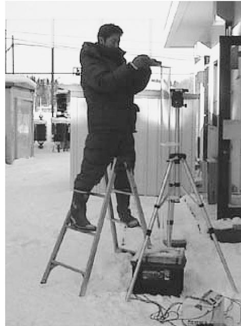
Fig. 4 System for terminal fall velocity measurement. Particles were allowed to fall in a cylinder. Their speed and size were measured when they passed through the two infrared rays of the sensors.
