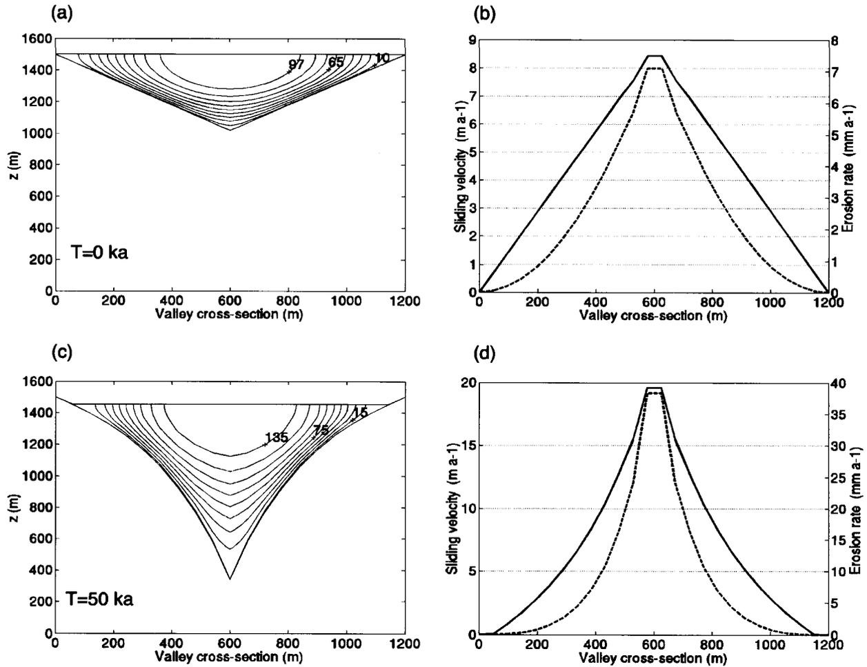
Fig. 2. (a) (c) Initial V-shaped valley and eroded valley obtained with the simplified model, velocity contours in  $\text{m a}^{-1}$ . (b) (d) Corresponding cross-glacier variation of sliding velocities (full line) and erosion rates (dotted line).
