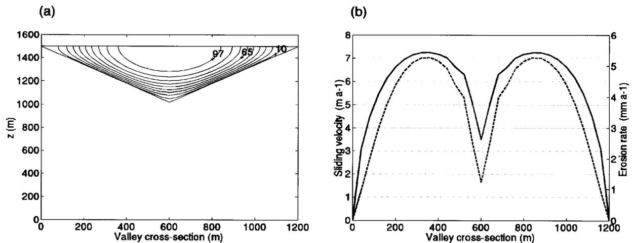
Fig. 3. (a) Initial V-shaped valley cross-section, velocity contours in  $\text{m a}^{-1}$ . (b) Corresponding cross-glacier variation of sliding velocities (full line) and erosion rates (dotted line).
