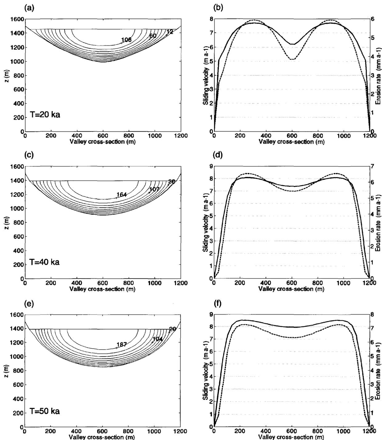
Fig. 4. (a) (c) (e) Model results for a simulation of glacial-valley development. Glacial-valley cross-section at three different time-steps, velocity contours in  $\text{m a}^{-1}$ . (b) (d) (f) Corresponding cross-glacier variation of sliding velocities (full line) and erosion rates (dotted line).
