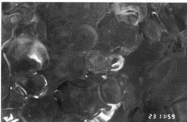
Fig. 10. Example of a moist snow surface ( $W_{vol,\%}=2.4\%$ ,  $\bar{d}=0.84$  mm and  $\delta_d=0.29$  mm).
