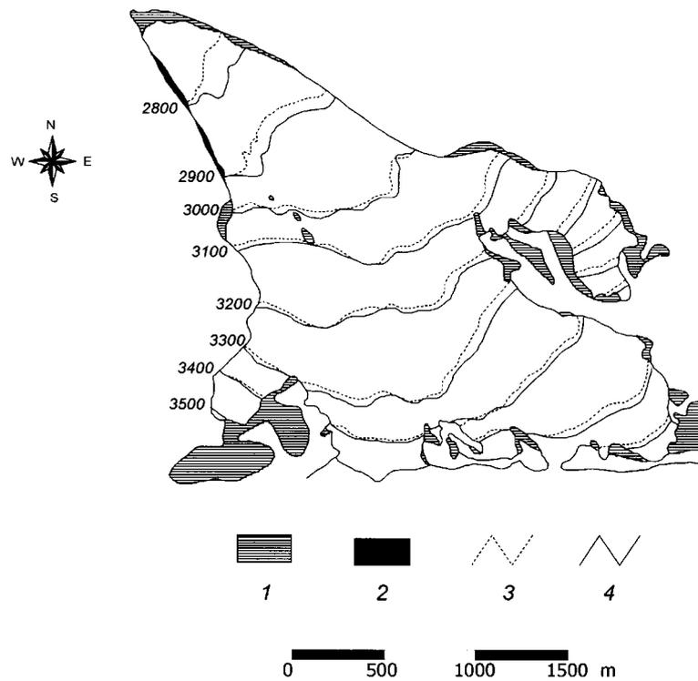
Fig. 5. Changes in the Djankuat Glacier 100 m interval contour lines and its boundaries in 1968–1999: 1 - areal loss; 2 - areal expansion; 3 - contour lines in 1968; 4 - contour lines in 1999.
