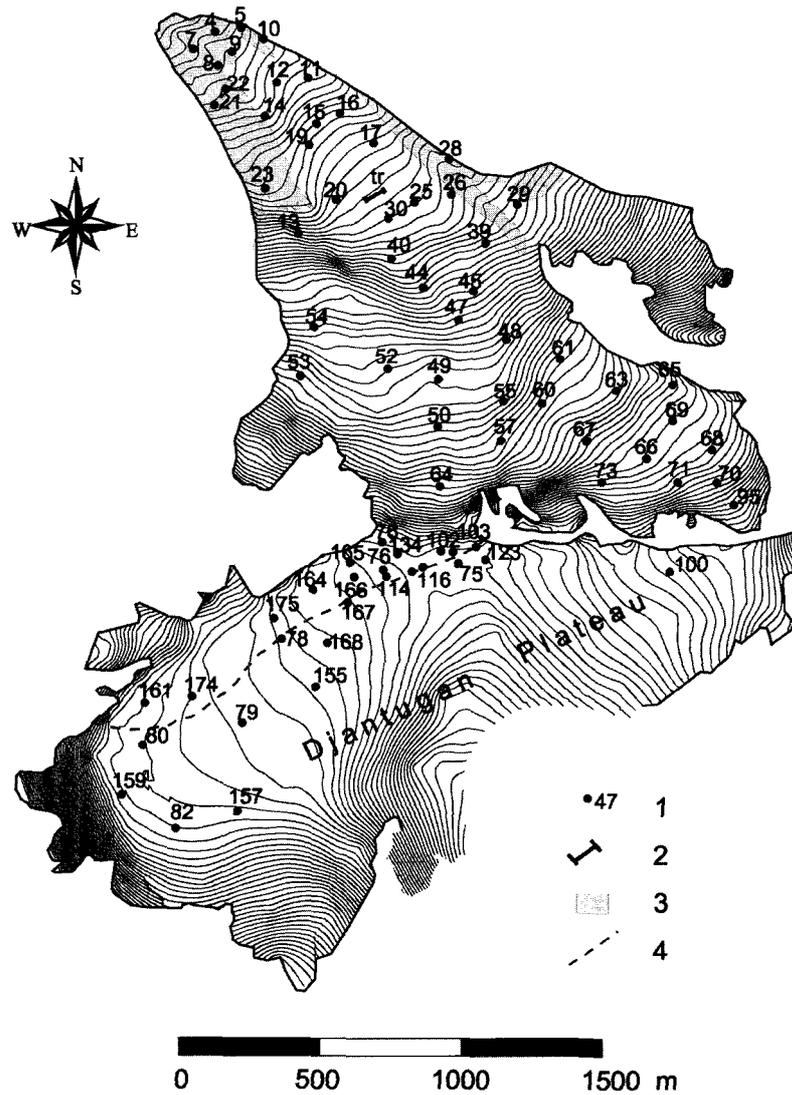
Fig. 3. b) Mass balance observational network at the Djankuat Glacier, for ablation measurements: 1 - ablation stakes and its numbers; 2 - reference cable; 3 - border of the debris cover on the glacier snout; 4 - border of the Djankuat Glacier catchment area on the Djantugan Plateau.
