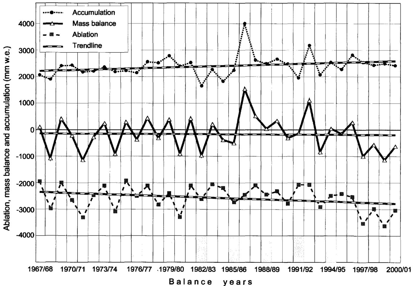
Fig. 4. Accumulation, ablation and mass balance fluctuations of the Djankuat Glacier during the 34-year-long period of direct measurements.
