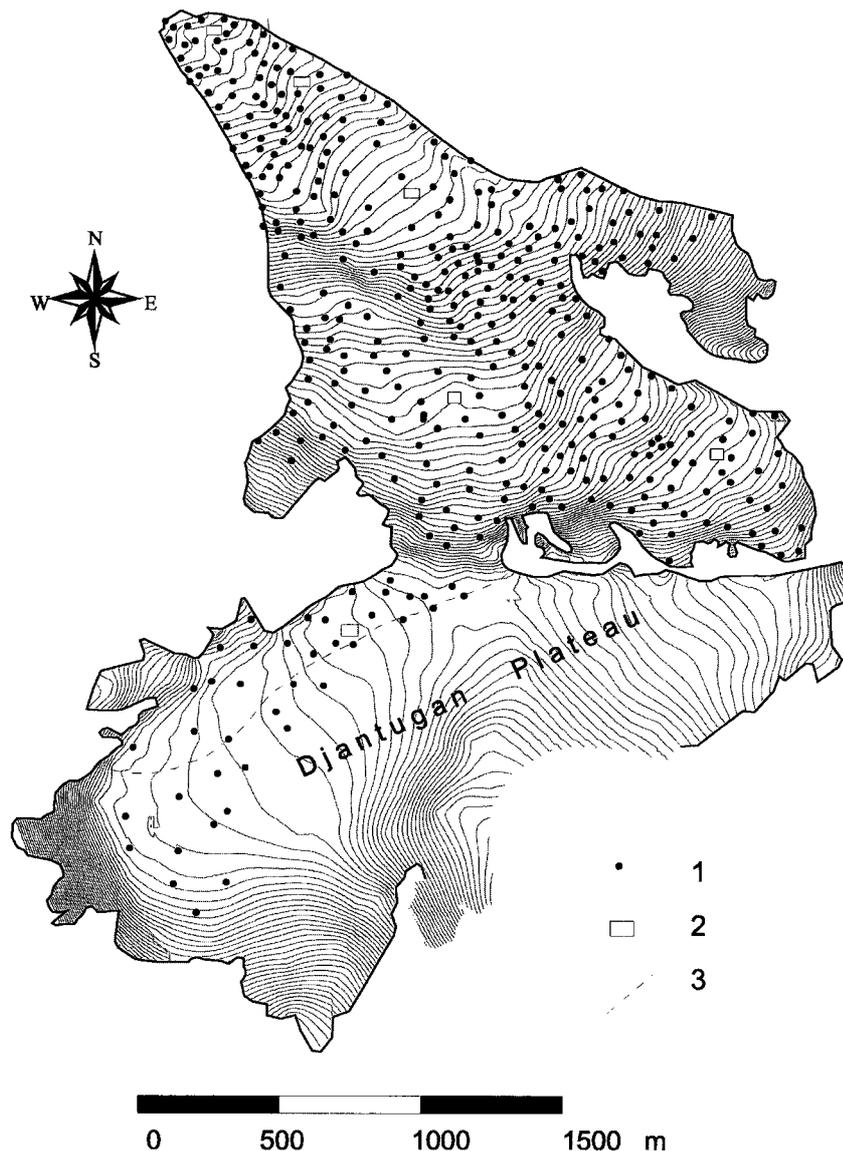
Fig. 3. a) Mass balance observational network at the Djankuat Glacier (status 1999 as an example), for accumulation measurements: 1 - measurement points of snow depth survey; 2 - snow pits for densimetry; 3 - border of the Djankuat Glacier catchment area on the Djantugan Plateau.
