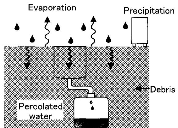
Fig. 2. Cutaway illustration of the lysimeter. Percolated water which does not evaporated descends through the debris layer and flows into a bottle from which it can be measured directly. Precipitation amount was observed by the tipping bucket. Evaporation amount was calculated by subtracting observed percolated water from observed precipitation amount.
