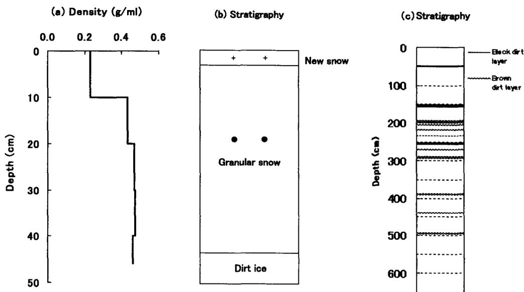
Fig. 12. a) Pit density, and stratigraphy at the drilling site observed by b) pit, and c) stratigraphy of ice cores.
