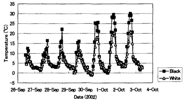
Fig. 10. Experiment of surface ground temperature by using black and white vinyl tapes at BC from 26 September to 3 October.
