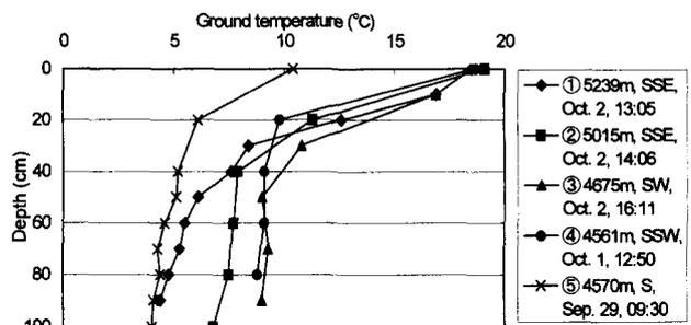
Fig. 11. Ground temperature profiles in moraines. Altitude, direction of ground surface, measured date and time at each site are described in the legend. Each location is; ①: upper, ②: middle, ③: lower parts of Tempete Glacier, ④: left lateral moraine near the outlet of Lugge Glacier, and ⑤: left lateral moraine of Thorthormi Glacier.
