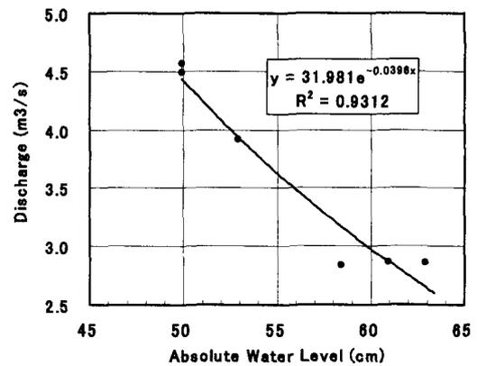
Fig. 7. Relationship between absolute water level and discharge.
