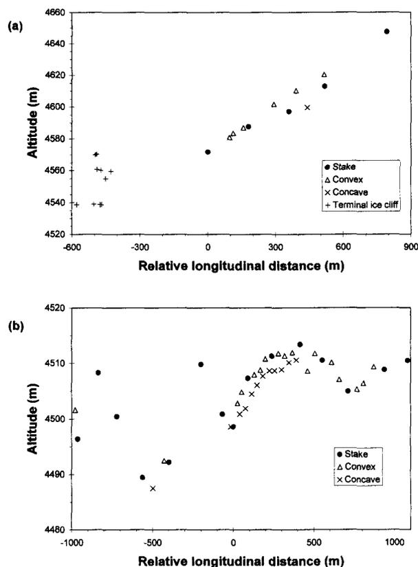
Fig. 9. Surface topography along the longitudinal line of (a) Lugge Glacier and (b) Thorthormi Glacier. The relative longitudinal distance refers to the cross point with the transversal survey line as positive to upstream.
