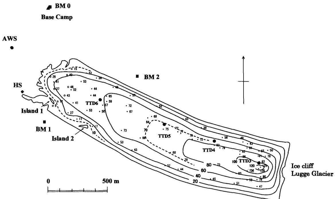
Fig. 4. Bathymetric map of Lugge Tsho. Small figures in the map represent depths of the lake measured at their surveyed points, the unit of which is meter.
