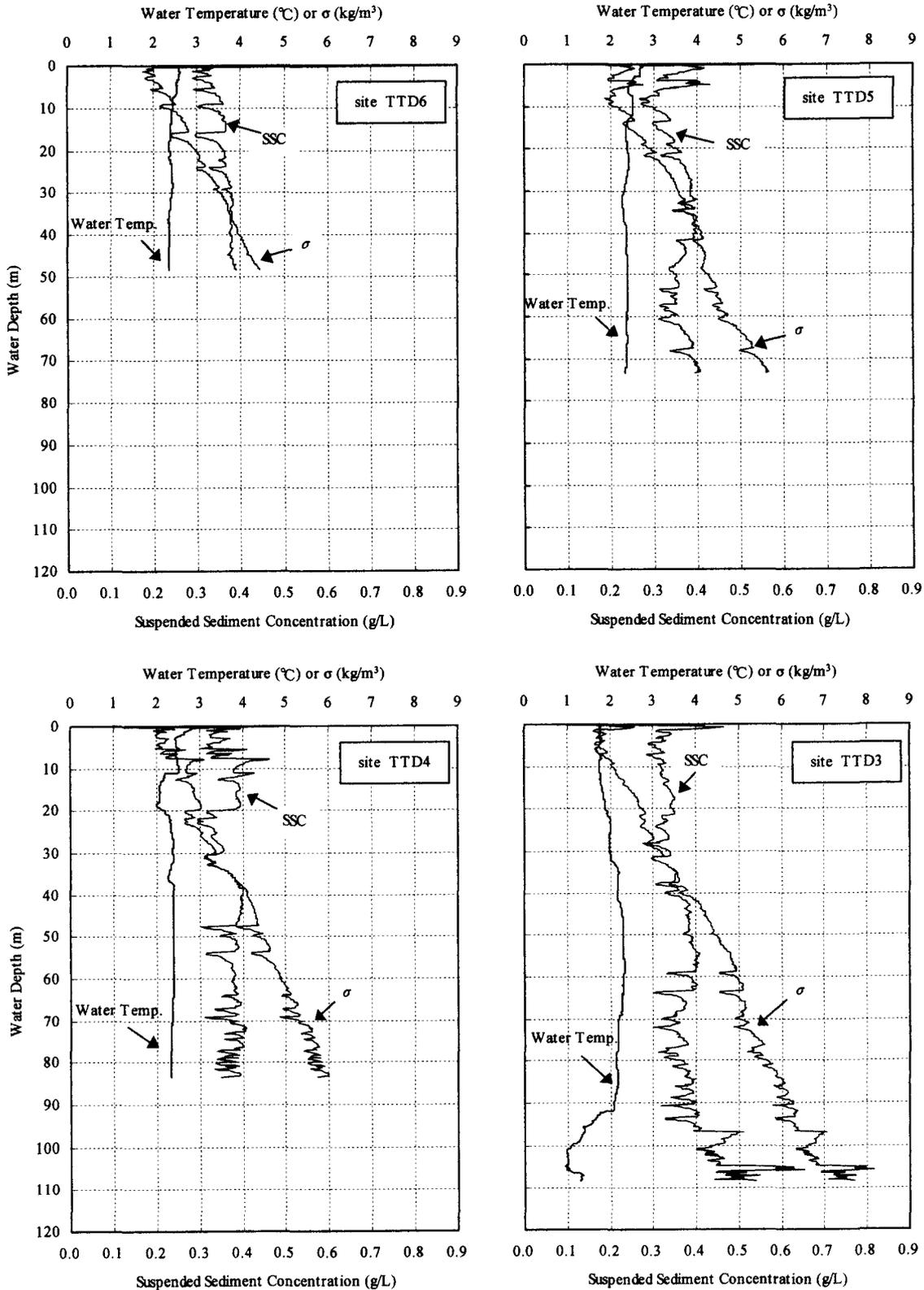
Fig. 5. Profiles of water temperature, suspended sediment concentration (SSC) and bulk density ( $\sigma$ ).
