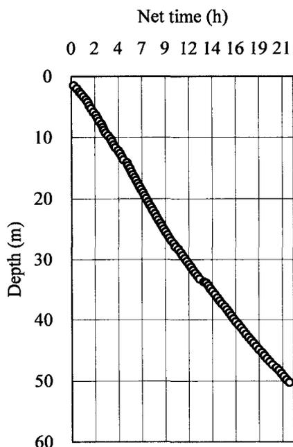
Fig. 4. Cumulative net drilling time (h) versus depth (m) at Mount Wrangell 2003.
