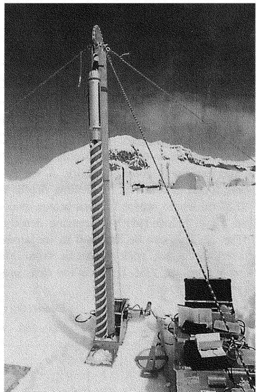
Fig. 3. The portable ice-core drilling system "Dokodemo Drill version 2" installed at the drilling site of the summit glacier of Mount Wrangell.
