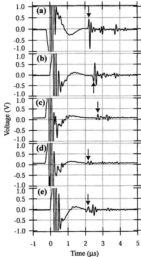
Fig. 5. Time series of received radio waves at five locations (a: Borehole; b: Kingcol 1; c: Kingcol 2; d: Kingcol 3; e: Kingcol 4 as shown in Fig. 3). Arrows indicate the reflection from the bedrock.
