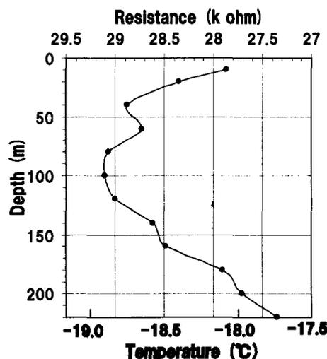
Fig. 11. Temperature profile of the wall of the borehole.
