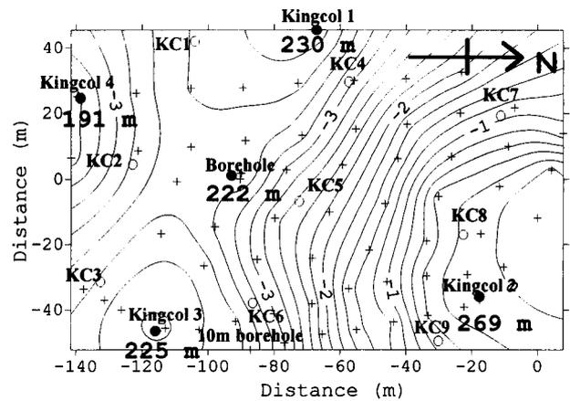
Fig. 3. Topographical map of the micro-relief at King Col (contour interval: 0.2 m). The contour line was drawn on the basis of our survey with the control point at the distances of (0, 0). Cross, open and solid dots indicate the surveyed points, snow stakes and the radar-echo sounding sites, respectively. Gothic 3 digit numbers indicate the thickness (m) of the ice sounded with the ice-penetrating radar.
