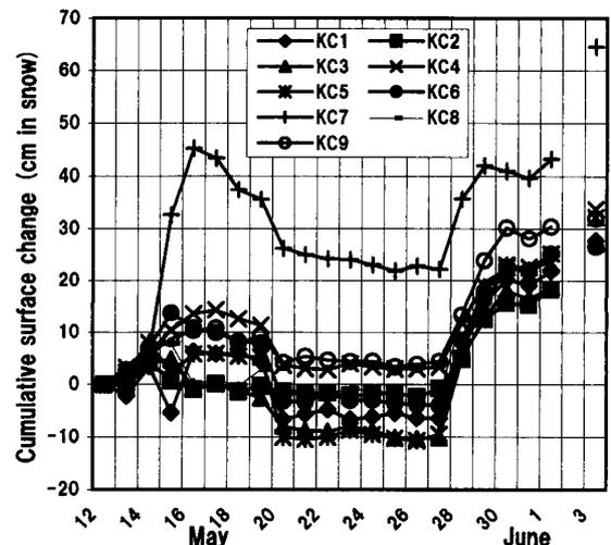
Fig. 4. Change of the snow surface during the drilling operation from May 12 to June 4. The stakes were installed inside the area shown in Fig. 3.
