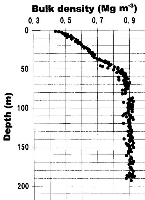
Fig. 9. Bulk density profile from the surface to the bottom of the borehole.
