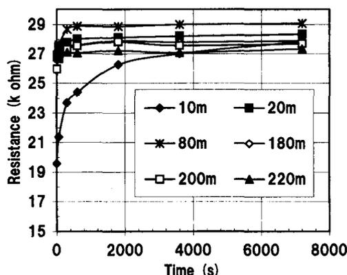
Fig. 10. Examples of the resistance (temperature) variations with time at six depths.
