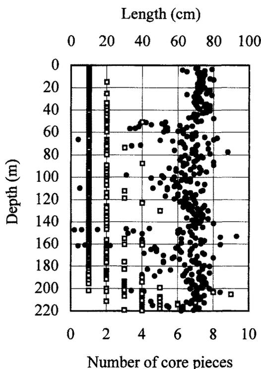
Fig. 8. Profiles of the length of each core (cm: black circles) and the pieces of the ice core obtained for each drilling run (open square).
