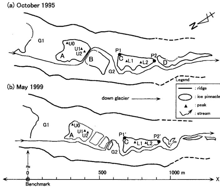
Fig. 2. Maps of the ice pinnacle zone in the Khumbu Glacier, (a) in 1995, (b) in 1999. A to D and U0 to L2 denote the ice pinnacles and peaks surveyed respectively. G1 and G2 are gaps in the ice pinnacle row. The scale bar also represents an abscissa of the coordinates positive downglacier. The origin of the coordinates is the benchmark on the crest of the right lateral moraine.
