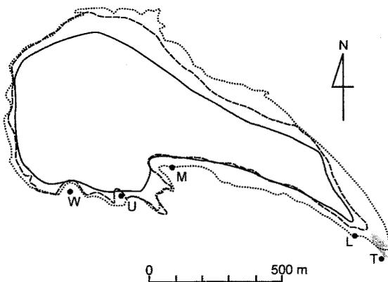
Fig. 2. Areal extents of Glacier AX010 surveyed in 1978 (dotted line; after Ageta *et al.*, 1980), 1996 (broken line; after Kadota *et al.*, 1997) and 1999 (solid line; this study). Solid circles denote the bench marks for survey. Hatched gray denotes a pond located near the terminus.
