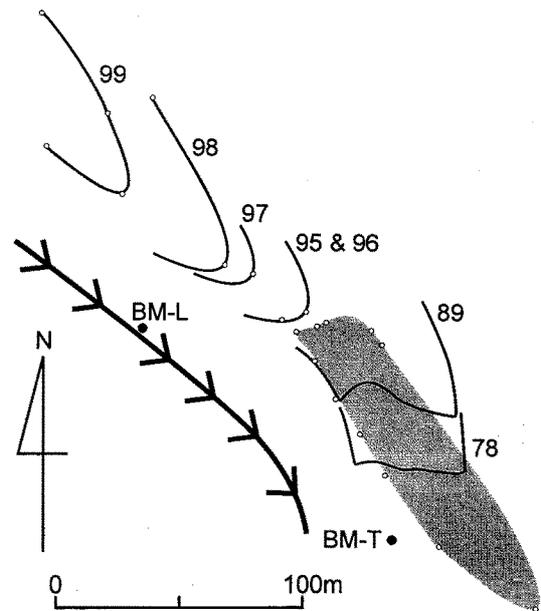
Fig. 3. Change in terminus periphery of Glacier AX010 surveyed in 1978 (after Ageta *et al.*, 1980), 1989 (after Kadota *et al.*, 1993) and every year from 1995 (this study). Peripheries in 1995 and 1996 are almost same position. Solid and open circles denote the bench marks for survey and surveyed points. Hatched gray denotes a pond located near the terminus. Thick solid line denotes ridge beside the glacier.
