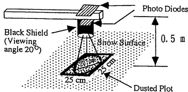
Fig. 1 Schematic diagram of the experimental procedures.
