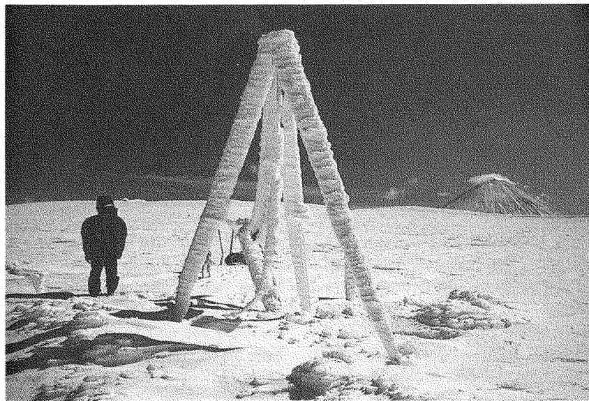
Fig. 5. Drilling tripod heavily coated with rime ice at Gorshkov crater, Ushkovsky Ice Cap.
