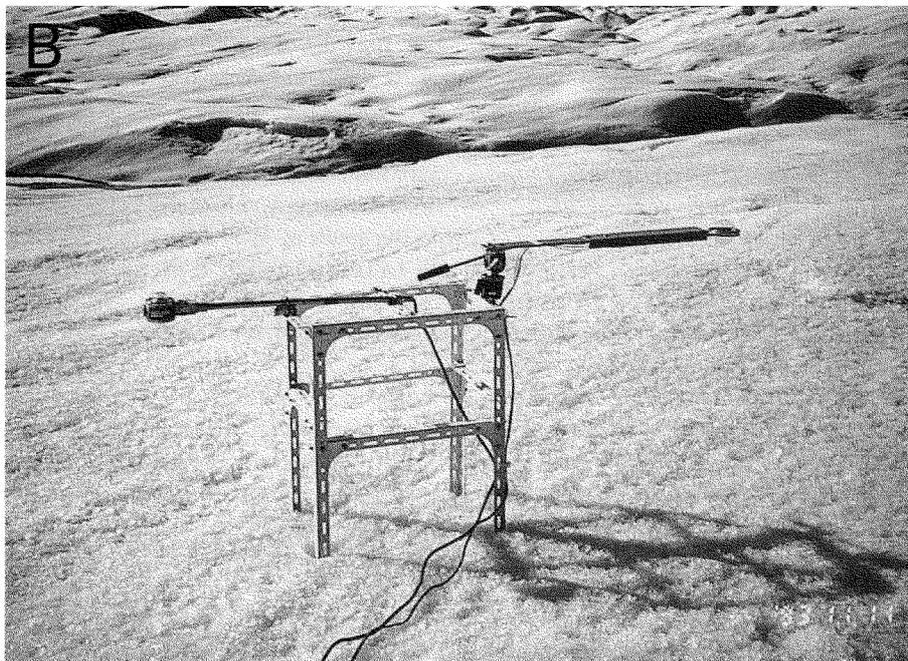
Fig. 6. Meteorological station at Moreno Glacier in November 1993. (A) A three-cup anemometer (left) and a hygro-thermometer covered with a ventilation pipe (right). (B) An albedo meter (left) and a net radiometer (right).
