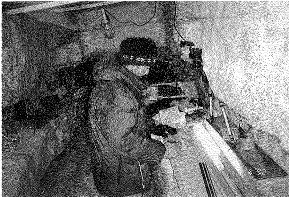
Fig. 8. Shallow ice coring with an electro-mechanical drill on Snøfjellaafonna.
