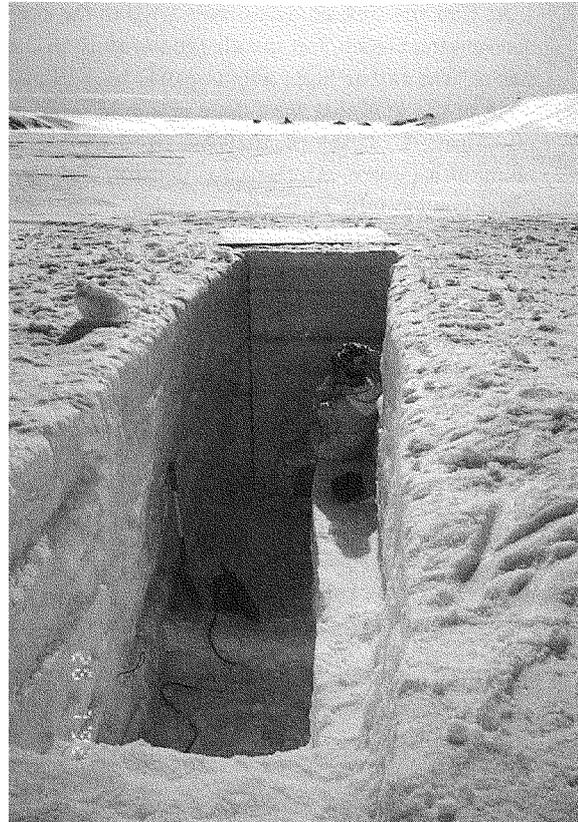
Fig. 9. Trench for core processing. Ice layers can be seen at intervals of several tens of centimetres.
