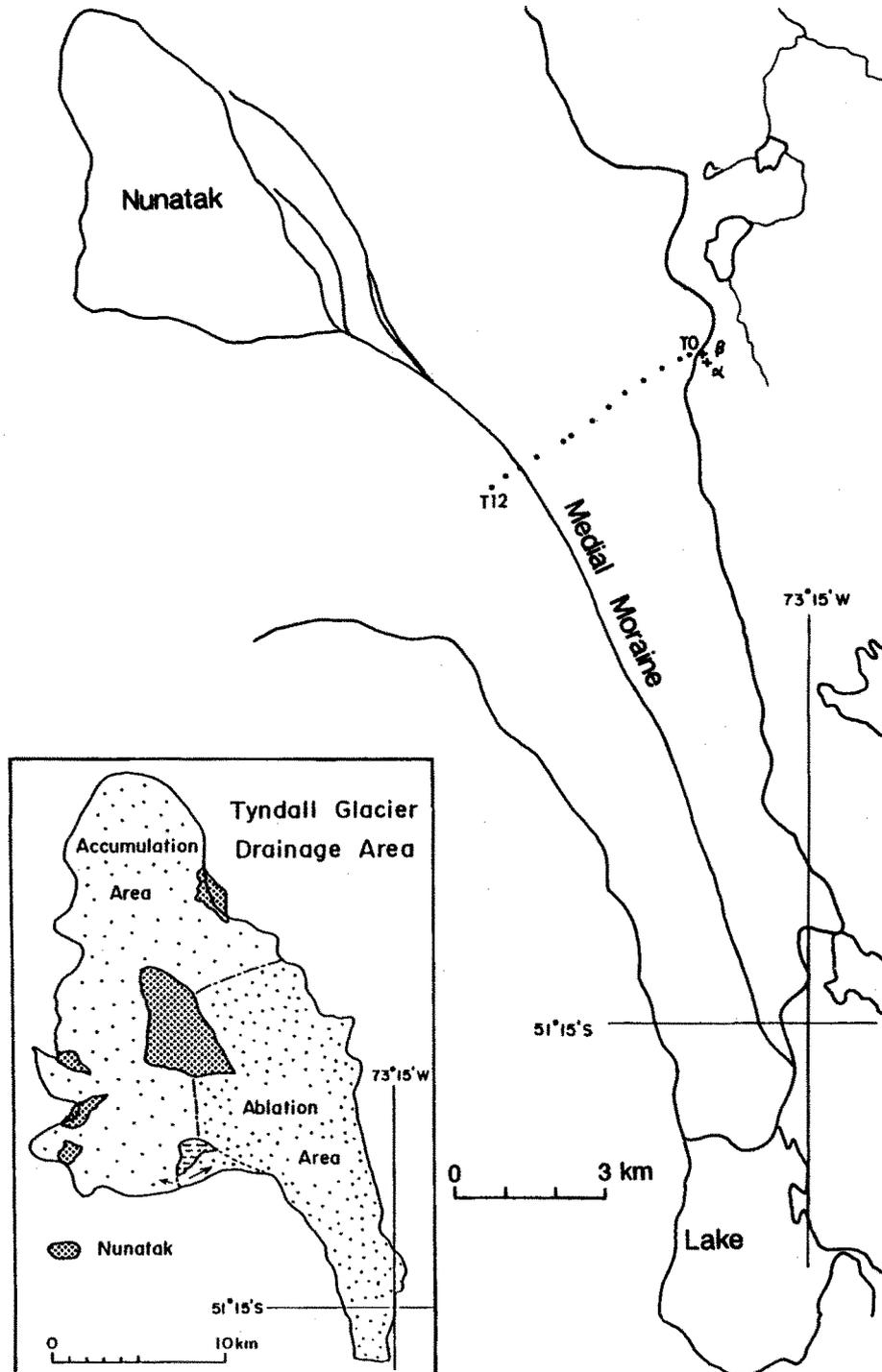
Fig. 1. Map of Tyndall Glacier (modified after Naruse et al., 1987). Surface level measurements were carried at the dotted points on the glacier.
