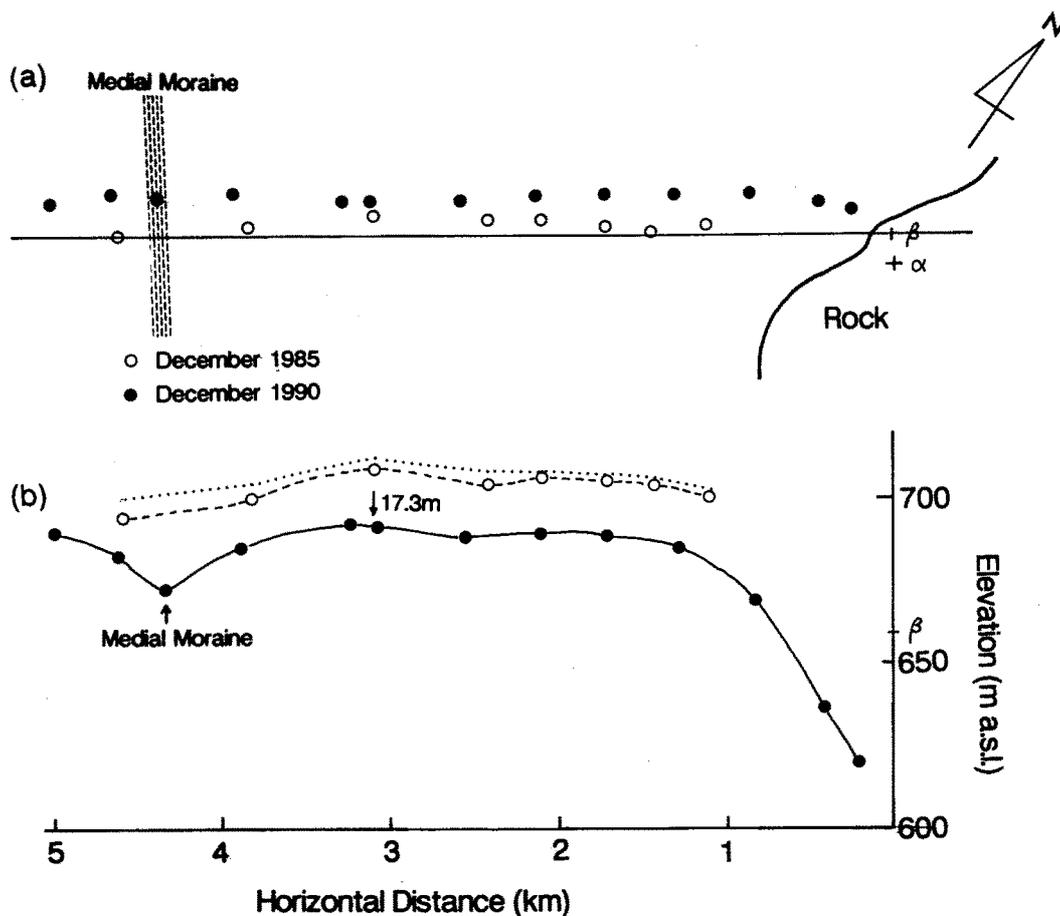
Fig. 3. (a) A plan view of survey points in 1985 and 1990. (b) Comparison of the surface profiles between 1985 and 1990 along survey lines. The dotted line shows an adjusted profile of the 1985 survey line (see text).
