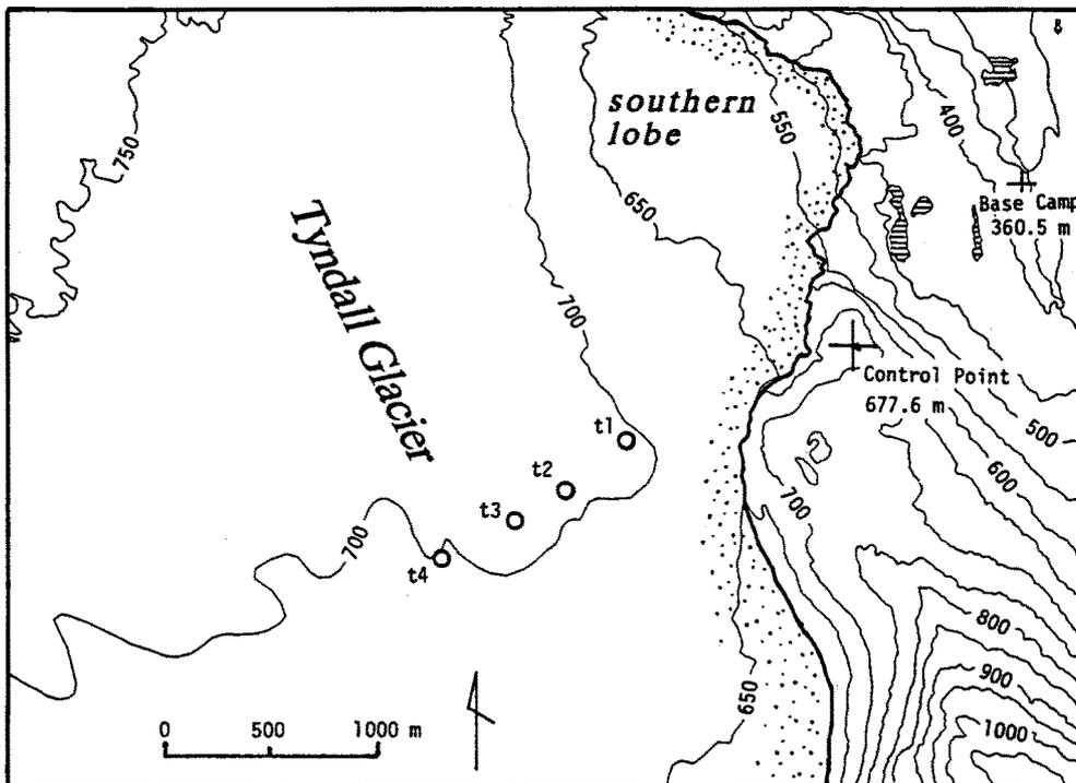
Fig. 4. Topographic map originally at a 1:25,000 scale produced from vertical aerial photographs taken in March 1975 by the Chilean Air Force. Digital mapping at contour intervals of 10, 25 and 50 m was done with a Zeiss planicomp P3. Contour lines are shown with an interval of 50 m. Control points were taken from the 1:100,000 topographic map "Rio Serrano" published by Instituto Geográfico Militar, Chile (1986). Some survey points in 1985 are shown by open circles.
