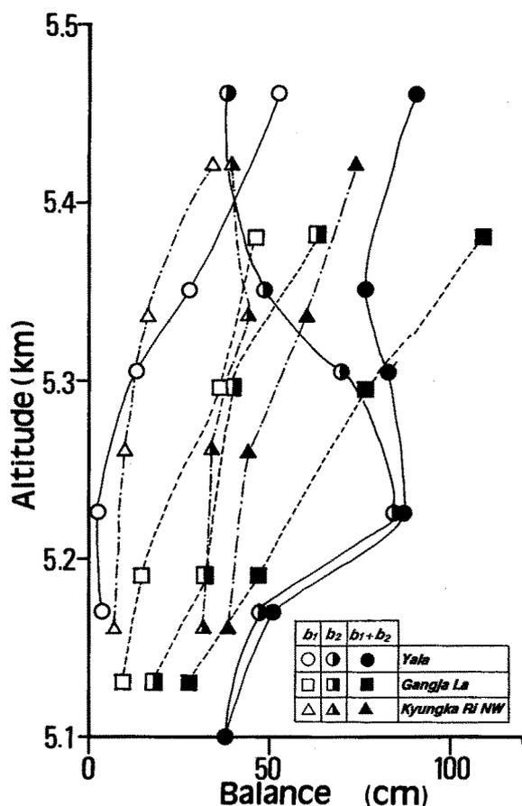
Fig. 9. Altitudinal changes of the values of the surface mass balances (equivalent to water) obtained from the snow profiles. The terms  $b_1$  and  $b_2$  indicate the surface mass balances during the monsoon season of 1990 and between the beginning of post-monsoon season of 1990 and May 1991, respectively.
