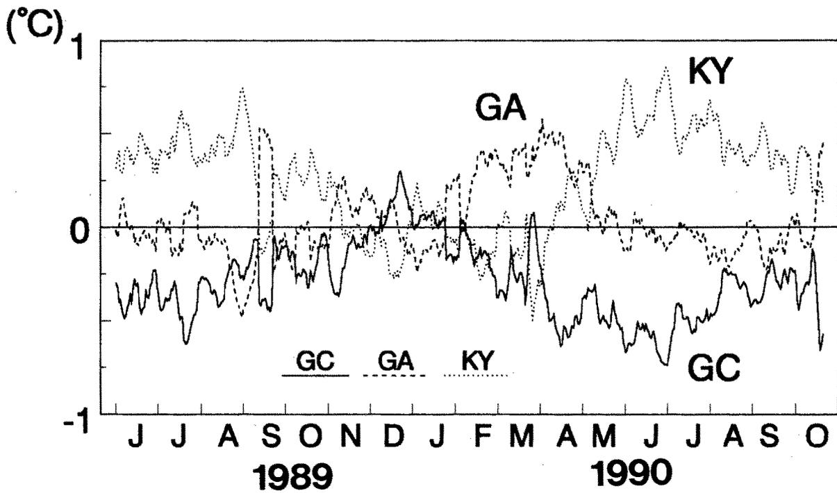
Fig. 5. Time-series of the 9 days running mean values of the air temperature anomalies from the average values of three stations. The air temperature at the Station KY (5140 m) was calibrated to the air temperature at the altitude of 5090 m, using a air temperature lapse rate of 6 °C/km.
