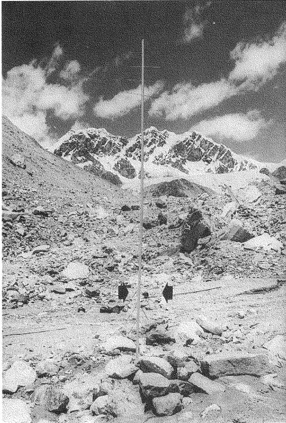
Fig. 2. Maximum snow depth meter at the Langtang Ri Base Camp (4942 m). Upper most bent bar denoted by the arrows indicates the level of maximum snow surface.
