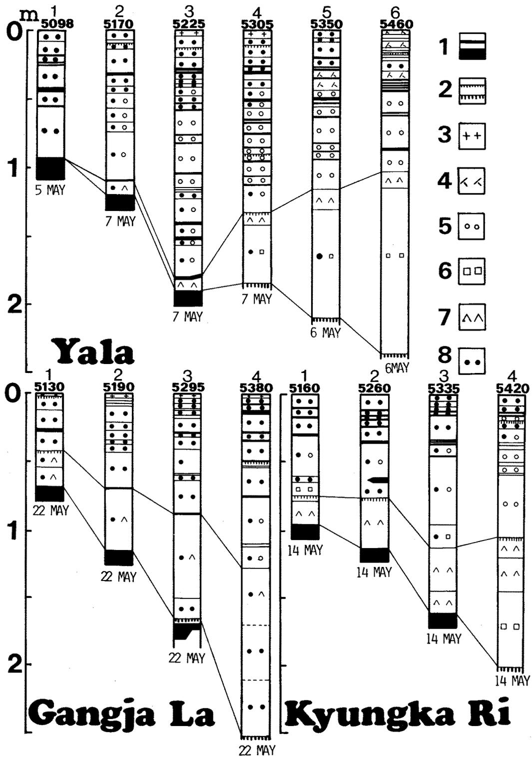
Fig. 8. Snow profiles excavated at each glacier on May, 1991. 1 : ice lens and ice layer, 2 : thin and thick dirt layers, 3 : new snow, 4 : lightly compacted snow, 5 : compacted snow, 6 : solid-type depth hoar, 7 : skeleton-type depth hoar, and 8 : granular snow.
