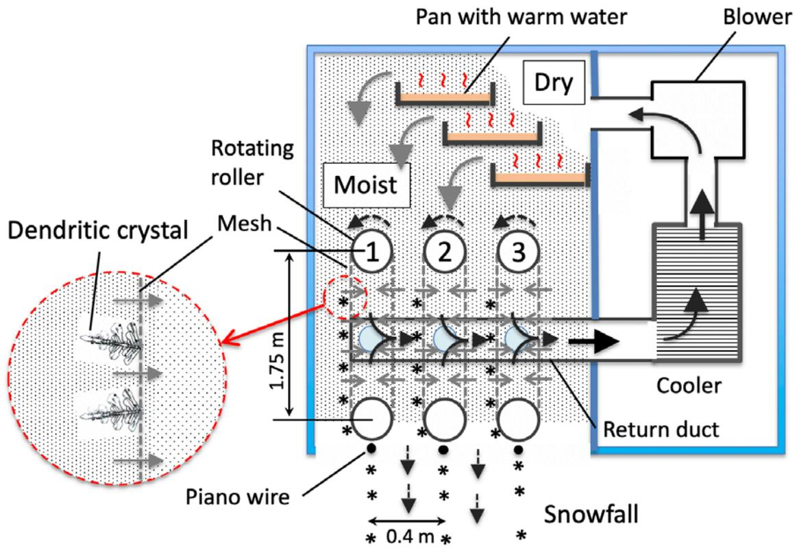
Fig. 2. Schematic of type A snowfall simulator with 3 units. There are 12 units in the simulator installed on the third floor.
