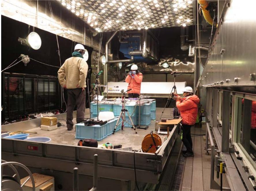
Fig. 6. Solar simulator. Solar radiation is controlled by the number of lamps that illuminate the object.
