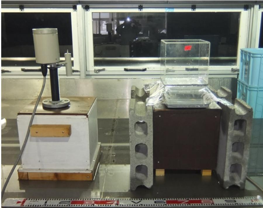
Fig. 5. Rain gauge (left) and balance with a square vessel (right).
