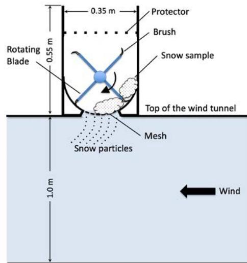
Fig. 8. Small snowfall machines used to sieve snow particles into the wind tunnel from the top window. Left: vibrational type, Right: rotating-brush type. Bottom figures show the snowfall machine schematics.
