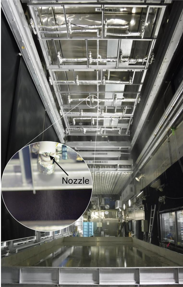
Fig. 4. Rainfall simulator installed on a carrier at the top of the first floor. Twenty-eight nozzles are laid out in 4 rows and 7 columns on the carrier. The large circle refers to the enlarged image of a nozzle shown in the small circle.
