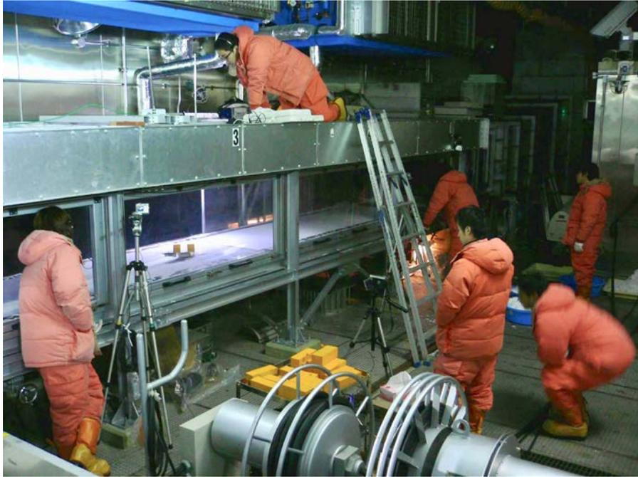
Fig. 7. Wind tunnel with a scale model of the object in the drifting snow layer. The test sections of both sides are comprised of transparent windows and all of the 2-m-wide front windows can be opened.
