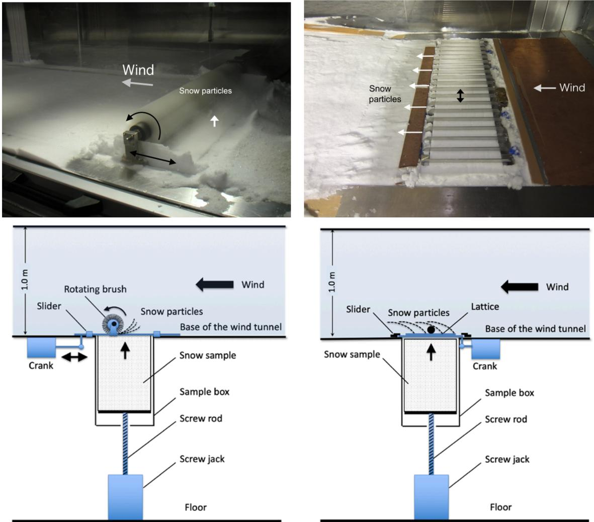
Fig. 9. Snow seeders in the wind tunnel. Left: rotating-brush type, Right: reciprocating type. Bottom figures show the snow seeder schematics. Dimensions of the sample box for both types are 0.2 m in length  $\times$  0.77 m in width  $\times$  0.3 m in depth.
