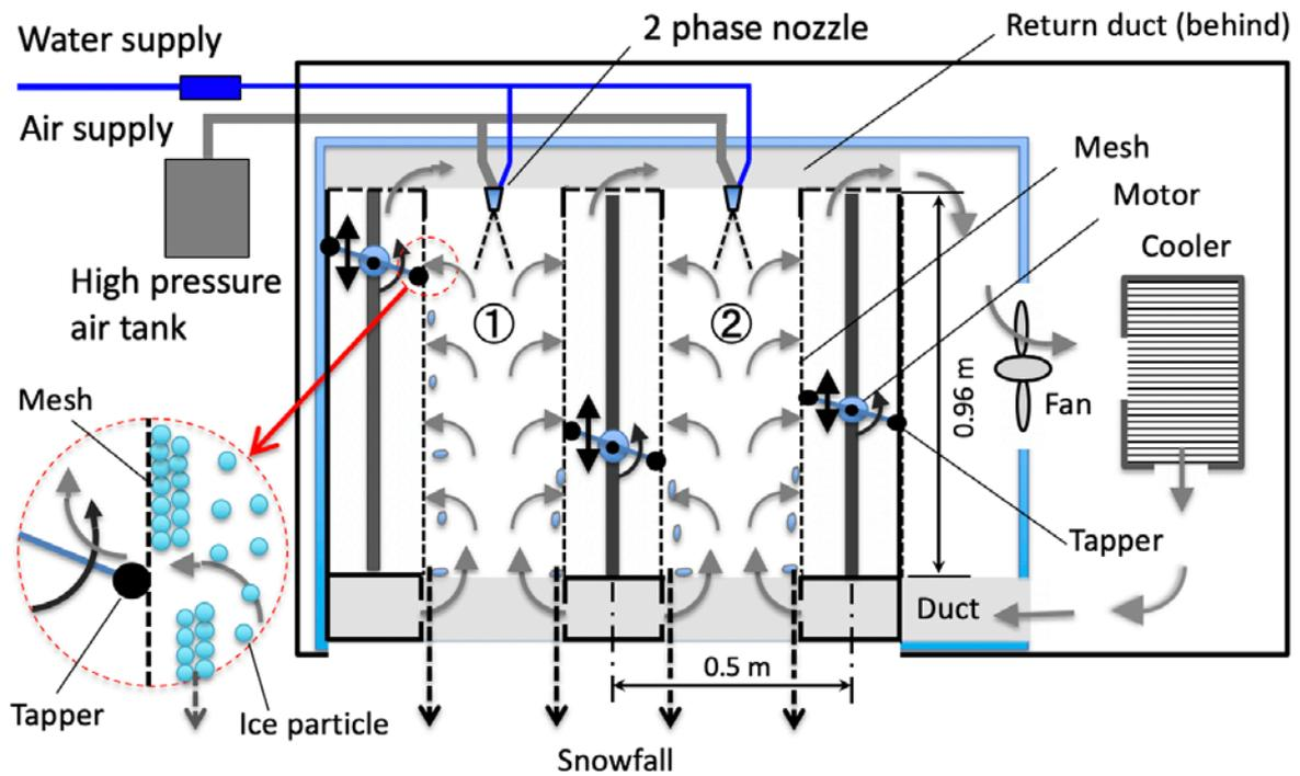
Fig. 3. Schematic of type B snowfall simulator with 2 units. There are 10 units in the simulator installed onto a carrier on the third floor.
