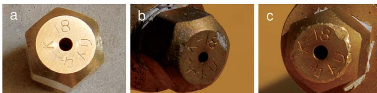
Fig. 4. Water jet nozzles (a) before the drilling and (b) after the drilling of BH1 and (c) BH4.
